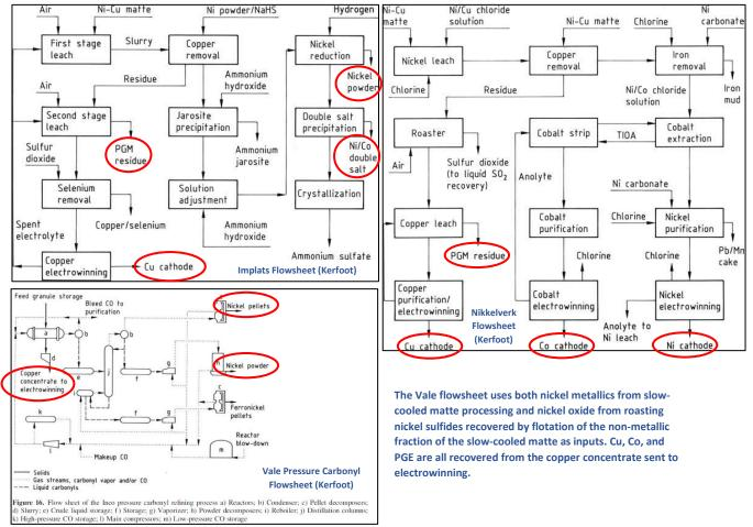
Although all of these flowsheets work, there are a number of pros and cons related to the feed material, location, etc. The complexity of choices of downstream processing of matte derives from the widely varying concentrate, and subsequently matte, compositions, as well as locational issues. Some of these include:
