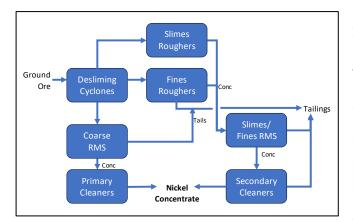
Other conceptually similar ores may contain numerous problematic minerals such as talc, hydrophobic magnesium silicates, and fibrous minerals which can cause significant flotation challenges and result in more complex flowsheets. The flowsheet left is of the Mt Keith concentrator (derived by the author from an Eriez paper<sup>xiii</sup>). Mt Keith encountered numerous problems on startup, and it took a dedicated longterm effort to achieve good process results.
