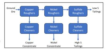
and purification circuit, a nickel recovery and purification circuit, and a third flotation step to remove high-sulfur materials from nickel tailings for separate tailings management to address potential acid generation issues that may not be a problem with lowsulfur ores. This practice is expected to become more common for higher sulfur ores due to increased stringency of environmental regulations.
