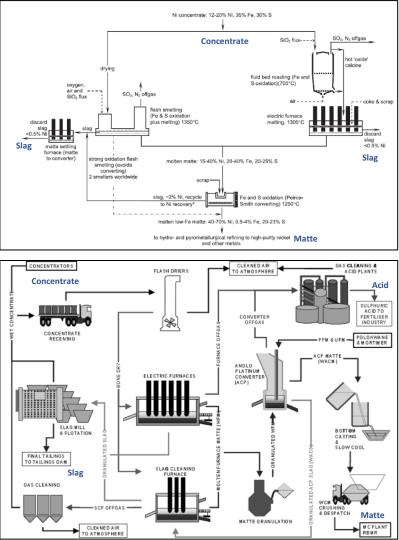
Physical processes for matte treatment including slow-cooling (multiple days), crushing, grinding, and flotation and/or magnetic separation are used in some installations to obtain multiple matte-derived products, achieving further Ni-Cu-PGE separation and allowing separate refining steps. Where such processes are not used, molten matte is often granulated by spraying into water.
